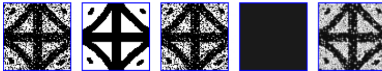
Fig. 2. Exemplar result of binary synthetic image denoising. From left to right: disturbed image, ground-truth and columns 3-5 are regression results of \varepsilon -SVR, SSVR^{cube} and our SSVR. Values lower than 0 or higher than 1 are adjusted to 0 or 1 respectively.
